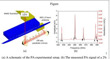
(a) A schematic of the PA experimental setup. (b) The measured PA signal of a 2% concentration of H₂S at a pressure of 100 mbar (black line) and the simulated
